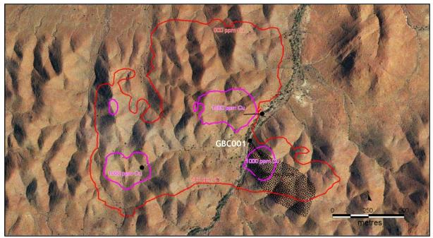
*Figure 2*. Gobbos prospect, defined by 500 ppm Cu-in-soil contour (red) with local highs > 1,000 ppm Cu (0.1% Cu) in purple and the Central Breccia (stippled). The location and trace of the three proposed drill holes is shown in black, the westernmost hole being vertical.
