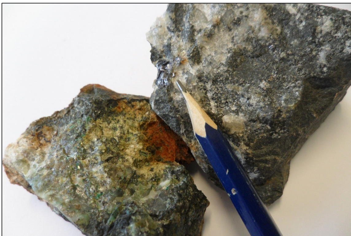
Figure 3. Chalcopyrite, malachite and molybdenite (at pencil tip) from brecciated basalt; eastern area, Gobbos prospect.
