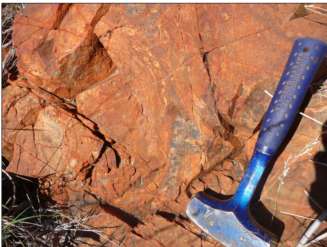
Figure 4. Brecciated inter-pillow matrix. Such zones suffer preferential disruption and are sites of more intense mineralisation. Gobbos prospect.
