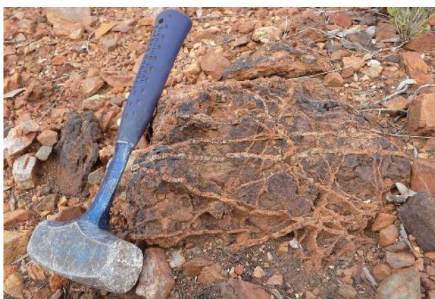
Figure 3. Intense quartz stockwork, Bridget prospect (sample P702426) with 0.62 g/t Au).
