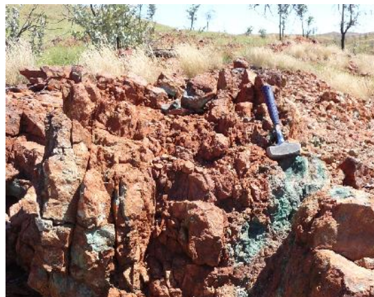
Figure 4. Wallabirdee Shear – shear zone with abundant malachite and hematite, 3.8 km west of Bridget prospect (sample P702461); 14.4% Cu.
