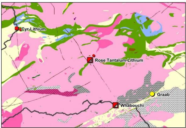
**Figure 3.** Summary geology of a portion of the James Bay region, Quebec, Canada, showing similarity of geological setting of Whabouchi and Lemare on the northern edge of a belt of metamorphosed greenstones (green and yellow) wrapping around a zone of high-grade granulite and migmatite (dark grey). (After Quebec Ministry of Energy and Natural Resources, 2016).
