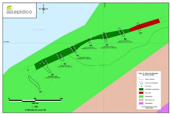
**Figure 5.** Trenching program at Lemare showing the six trenches channel sampled as per Table 1.
