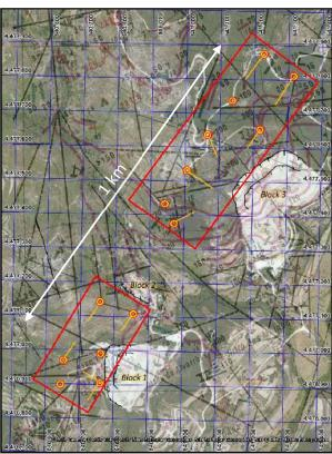
**Figure 3.** Proposed location of diamond drill holes covering the Block 1 and Block 3 targets at the Gonçalo lepidolite mine. Each site will include a vertical hole plus angled holes as shown.
