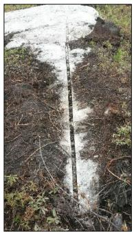
**Figure 3.** Channel sample across SW Extension spodumene pegmatite.
