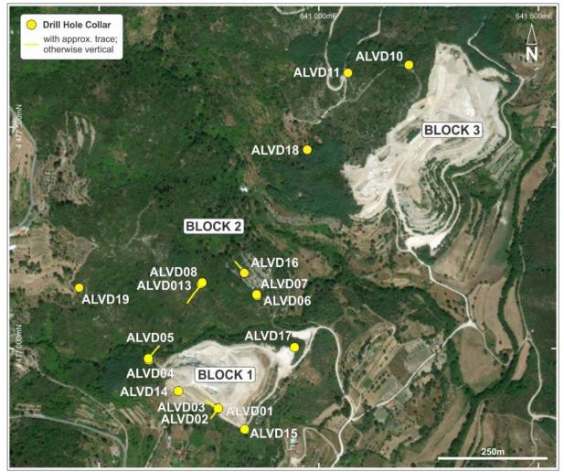
**Figure 1**. The lithium pegmatites at Alvarrões have been confirmed by drilling to extend at least 900 m along strike (ALVD19 to ALVD10) and 500 m down-dip (ALVD15 to ALVD19). All holes intersected mineralised lepidolite-bearing pegmatites. The system remains open in all directions.
