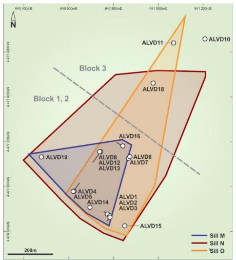
*Figure 2.* Plan view of the wireframes of the three mineralised pegmatite sills at Alvarrões used in the Mineral Resource estimation, before being cut to topography.
