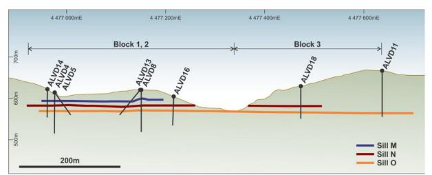
*Figure 3.* Long-section through the Alvarrões lithium deposit, showing continuity of the three lepidolite-bearing pegmatite sills used in the Mineral Resource estimate and separation by topography into the Block 1 & 2 and Block 3 domains. Note, sill thickness schematic; varies from 0.5 m to over 4.0 m.
